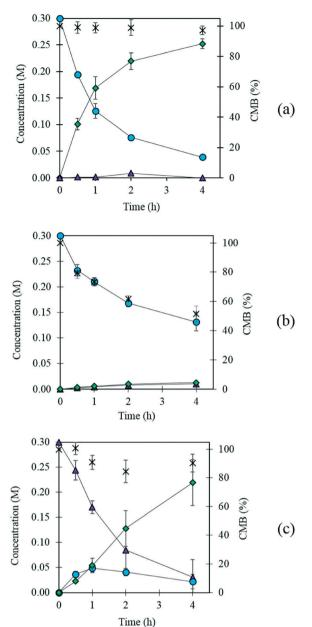
Fig. 2 (a) The oxidation of FF in the presence of a 1 wt% AuPd/ Mg(OH)<sub>2</sub> catalyst and (b) in the absence of a catalyst. (c) corresponds to the oxidation of furfuryl alcohol in the presence of a 1 wt% AuPd/ Mg(OH)<sub>2</sub> catalyst. Reaction conditions: 303 K, p: 3 bar O<sub>2</sub>, NaOH: FF equivalents: 1, reaction volume (10 mL), catalyst (91.1 mg). Key: FF O, FOH  $\triangle$ , FA  $\diamondsuit$ , carbon mass balance (CMB)  $\times$ .
