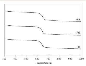
Fig. 4 TGA of (a) fresh  $AuPd/Mg(OH)_2$  catalyst, (b) used  $AuPd/Mg(OH)_2$  tested at 303 K and (c) used  $AuPd/Mg(OH)_2$  tested at 343 K. Samples were heated at a ramp rate of 5 K min<sup>-1</sup> in air.
