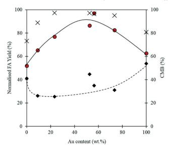
Fig. 7 Oxidation of FF over a series of mono- and bi-metallic catalysts containing Au and Pd supported on Mg(OH)2. Normalised FA yield corresponds to the FA yield expected assuming the total metal loading is equal to 1 wt%. Reaction conditions: 0.3 M FF, 303 K, p: 3 bar O<sub>2</sub>, NaOH: FF equivalents: 1, 10 mL reaction volume, 91.1 mg catalyst. FA yield at 0.5 h ◆, FA yield at 4 h ●, carbon mass balance at 4 h (CMB)
