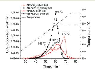
Fig. 7 TPO curves of the spent samples obtained after the short and the long term (stability) tests. Short tests: full symbol, long test: empty symbol. CO2 production was measured by QMS and temperature was ramped during TPO to 600 °C or 750 °C after the short or stability tests, respectively.
