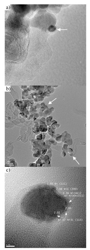
Fig. 6 TEM images taken after short term catalytic tests on (a) Ni/ZrO<sub>2</sub> and (b) Na-Ni/ZrO<sub>2</sub>. (c) HRTEM image of a single Ni particle at the end of a nanotube in the spent Na-Ni/ZrO<sub>2</sub>.
