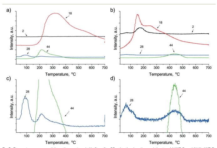
Fig. 3 Temperature programmed desorption spectrum in He flow after CO pulse chemisorption carried out on (a) Ni/ZrO<sub>2</sub> and (b) Na-Ni/ZrO<sub>2</sub> and the corresponding enlarged 28 (=CO) and 44 (=CO<sub>2</sub>) signals of (c) Ni/ZrO<sub>2</sub> and (d) Na-Ni/ZrO<sub>2</sub>. Note that the second peak in the m/z = 28signals corresponds only to the fragmentation of CO2 in both cases.
