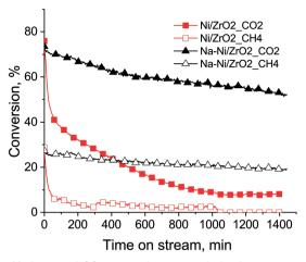
Fig. 8 Methane and CO<sub>2</sub> conversion curves during long term stability run on both samples. CH<sub>4</sub>: empty symbols, CO<sub>2</sub>: full symbols. Conditions: after reduction at 750 °C/0.5 h cooling to T = 675 °C in He, then DRM with  $CH_4: CO_2: Ar = 68: 31:1$  mixture, 120 L  $h^{-1}$   $g_{cat}^{-1}$ .
