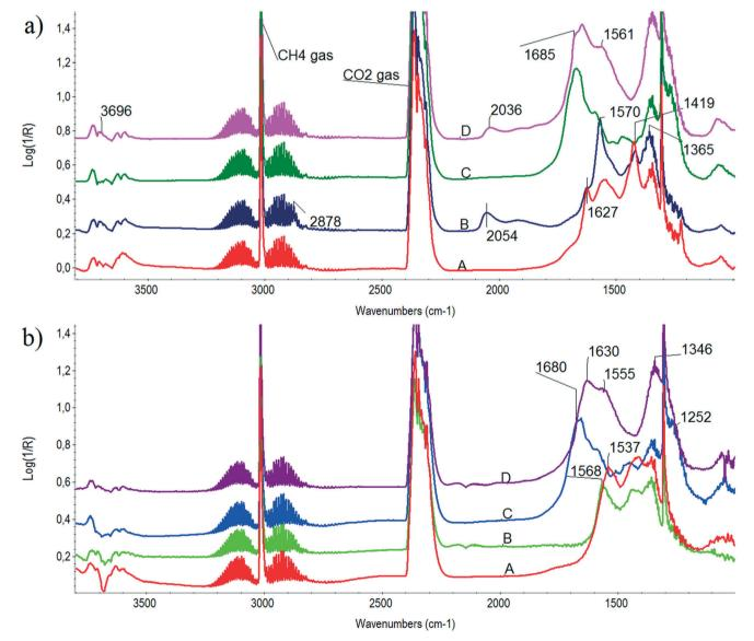
Fig. 4 DRIFTS spectra obtained in the presence of CH<sub>4</sub>: CO<sub>2</sub> = 70:30 DRM flow at (a) 300 °C and (b) 500 °C. Curve A: ZrO<sub>2</sub> support, B: Ni/ZrO<sub>2</sub>, C: Na-ZrO<sub>2</sub> support, D: Na-Ni/ZrO<sub>2</sub>.
