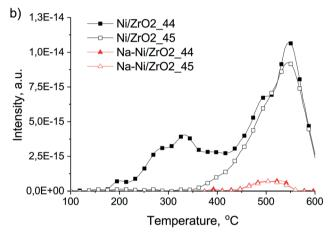
Fig. 10 TPO experiments in the circulation system after labeled DRM reaction carried out via the (a) ramp-hold manner and (b) isothermal manner at 600 °C. <sup>12</sup>CO<sub>2</sub>: full symbols, <sup>13</sup>CO<sub>2</sub>: empty symbols. The original measured integral signals are differentiated to get peakshaped curves.
