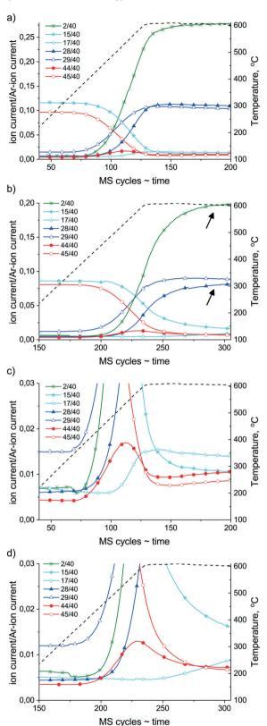
Fig. 9 Ramp-hold type dry reforming reaction with a  $^{13}\text{CO}_2$ :  $^{12}\text{CH}_4=1$  mixture in the closed loop circulation system on (a) Ni/ZrO $_2$  and (b) Na–Ni/ZrO $_2$ . (c) Enlargement of low intensity signals of spectrum "a" and (d) enlargement of low intensity signals of spectrum "b". Conditions: ~25 mbar each reactant ( $^{12}\text{CH}_4$  contains 2% Ar), temperature ramp with 10 °C min $^{-1}$  up to 600 °C then isothermal 30 min at 600 °C. 1 MS cycle = 26 s.
