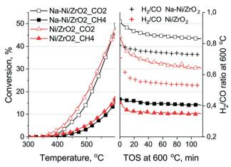
Fig. 5 Methane and CO<sub>2</sub> conversion curves and the H<sub>2</sub>/CO ratios during a short term catalytic run on both samples. CH<sub>4</sub>: full symbols,  $CO_2$ : empty symbols. Conditions: temperature ramp in  $CH_4$ :  $CO_2$ : Ar = 68:31:1 mixture, 120 L h $^{-1}$  gcat  $^{-1}$ , at a 10  $^{\circ}\text{C}$  min  $^{-1}$  rate to 600  $^{\circ}\text{C}$  and then isothermal 120 min hold time.
