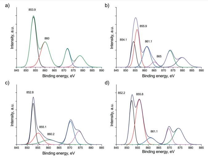
Fig. 2 Ni 2p region measured by XPS after calcination at 600 °C on (a) Ni/ZrO<sub>2</sub> and (b) Na–Ni/ZrO<sub>2</sub> and after reduction at 600 °C on (c) Ni/ZrO<sub>2</sub> and (d) Na–Ni/ZrO<sub>2</sub>. Fitted curves are shown.
