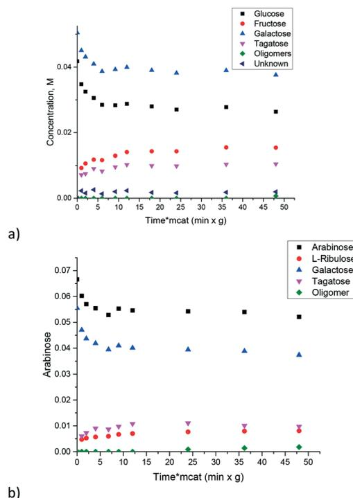
Fig. 10 Isomerization of sugar mixtures over the  $(\text{MgO})_{0.8}(\text{Al}_2\text{O}_3)_{0.2}$  catalyst for a) galactose–glucose and b) galactose–arabinose mixtures. Reaction conditions: temperature = 110 °C, calcination temperature = 680 °C,  $m_{\text{cat}} = 0.2 \text{ g}$ , 5 bar and 1000 rpm.
