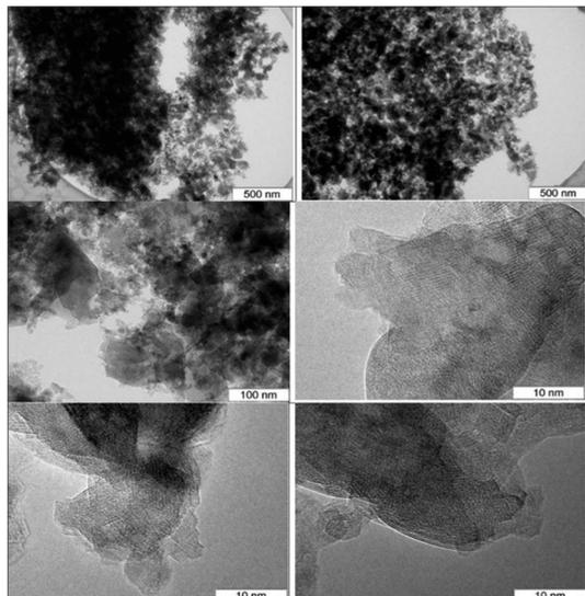
Fig. 13 TEM of the  $(\text{MgO})_{0.7}(\text{Al}_2\text{O}_3)_{0.3}$  catalyst.
