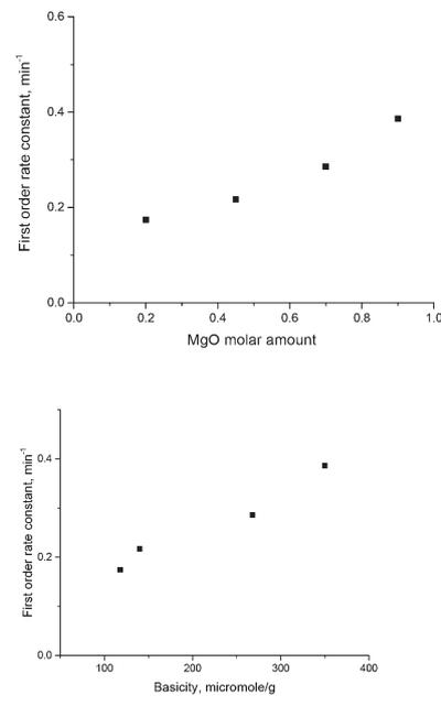
Fig. 9 Galactose isomerization first order rate constant vs. a) molar Mg content and b) basicity of magnesium aluminates. Reaction conditions: 110 °C,  $m_{\text{cat}} = 9.2 \text{ g}$ , 5 bar, 1000 rpm and calcination temperature = 680 °C.
