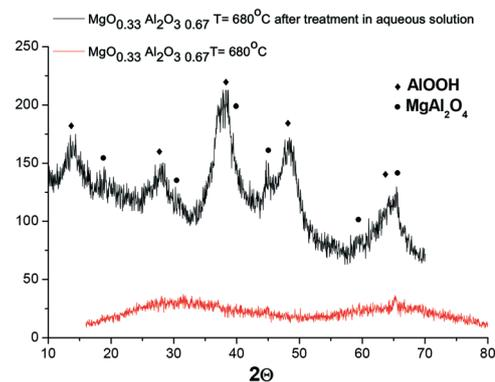
**Fig. 12** XRD diffractogram of (MgO)<sub>0.33</sub>(Al<sub>2</sub>O<sub>3</sub>)<sub>0.67</sub> calcined at 680 °C prior to and after hydrothermal treatment at 110 °C for 2.5 h in galactose solution.
