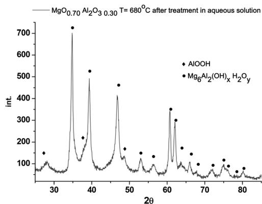
**Fig. 11** XRD data for the (MgO)<sub>0.7</sub>(Al<sub>2</sub>O<sub>3</sub>)<sub>0.3</sub> catalyst calcined at 680 °C and hydrothermally treated at 110 °C for 2.5 h in galactose solution.
