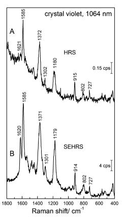
Fig. 10 (A) Hyper Raman spectrum of crystal violet dye and (B) surface enhanced hyper Raman spectrum of crystal violet in the local field of silver nanostructures. Excitation: 1064 nm (A and B), photon flux density:  $6.8 \times 10^{27} \text{ photons cm}^{-2} \text{ s}^{-1}$  (A) and  $1.4 \times 10^{27} \text{ photons cm}^{-2} \text{ s}^{-1}$  (B), acquisition time: 8 min (A) and 1 min (B), crystal violet concentration:  $1 \times 10^{-3}$  M (A) and  $1 \times 10^{-5}$  M (B).
