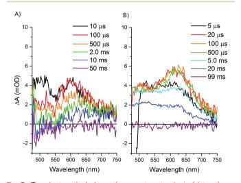
Fig. 7 Transient optical absorption spectra at selected later times. Samples contained 200 mM sodium ascorbate and were excited at 460 nm and detected with a fiber laser. (A) Ru-ApoFld-CoBF<sub>2</sub> spectra, (B) Ru-Fd-CoBF<sub>2</sub> spectra.
