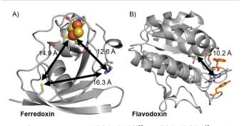
Fig. 2 Crystal structures of (A) Fd (1A70)<sup>25</sup> and (B) Fld (1CZL)<sup>42</sup> proteins with distances between possible binding sites for catalysts, PSs, and native redox cofactors. The closest relative distances between catalyst and PS binding sites and redox cofactors are indicated on the figure.
