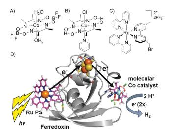
Fig. 1 (A–C) Catalysts and photosensitizers used in the current study. Cobaloxime catalysts (A) Co(dmgBF $_2$ ) $_2$ ·2H $_2$ O (CoBF $_2$ ) and (B) Co(dmgH) $_2$ pyCl (CoPy) and (C) ruthenium photosensitizer (Ru PS), [Ru(4-CH $_2$ Br-4'-CH $_3$ -2,2'-bpy)(bpy) $_2$ ]·2PF $_6$ . (D) Photocatalytic hydrogen production scheme in Ru–Fd–CoBF $_2$  biohybrid utilizing electron transfer through the native Fd [2Fe–2S] cluster (1A70).25
