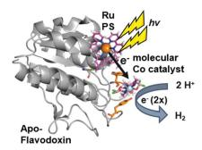
Fig. 3 Scheme for hydrogen production in Ru–ApoFld–Co biohybrid complexes with electron transfer directly from the Ru PS to the Co catalyst (1CZL).<sup>42</sup> The protein is proposed to refold around the catalyst in the FMN binding pocket.
