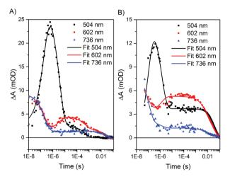
Fig. 6 Kinetic fits of transient optical kinetic data for the (A) Ru-ApoFld-CoBF<sub>2</sub> and (B) Ru-Fd-CoBF<sub>2</sub> biohybrids with 200 mM sodium ascorbate using a global kinetic fitting routine at three wavelengths (504 nm (black), 602 nm (red), and 736 nm (blue)) in Origin Pro 9.1. The data sets were fit with four-exponential decay functions from 10-50 ns to 100 ms.
