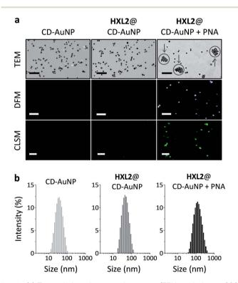
Fig. 3 (a) Transmission electron microscopy (TEM, scale bar =200 nm, arrows indicate aggregated particles), dark-field microscopy (DFM, scale bar  $=20~\mu m$ ) and confocal laser scanning microscopy (CLSM, scale bar  $=10~\mu m$ ) of CD-AuNP (7 nM) and HXL2@CD-AuNP (0.56  $\mu M/7$  nM) without or with PNA (70  $\mu M$ ). (b) Dynamic light scattering of CD-AuNP (7 nM) and HXL2@CD-AuNP (0.56  $\mu M/7$  nM) without or with PNA (30  $\mu M$ ).
