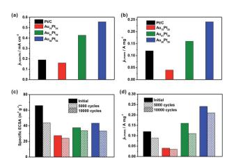
Fig. 5 Oxygen reduction performances of three types of AuPt@Pt bimetallic catalysts with different thicknesses of Pt dendritic branches relative to a commercial Pt/C catalyst. (a) Specific and (b) mass activities of the catalysts at 0.9  $V_{\rm RHE}$ . (c) Specific ECSAs and (d) mass activities (at 0.9  $V_{\rm RHE}$ ) of the catalysts before and after accelerated durability testing. The colour scheme applies to all panels.
