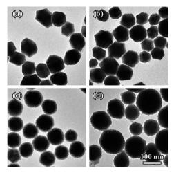
Fig. 4 TEM images of the Au–Pt bimetallic NCs that were prepared using the standard procedure, except for variation in the introduced amount of  $K_2PtCl_4$  (1 mM): (a) 0.5 mL, (b) 1.0 mL, (c) 2.0 mL and (d) 3.0 mL.
