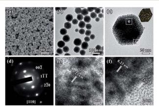
Fig. 1 (a and b) SEM and TEM images of the porous rhombic dodecahedral AuPt@Pt bimetallic NCs. (c and d) A TEM image and corresponding SAED pattern of one individual NC. (e and f) HR-TEM images of the two regions of the NC shown in (c).
