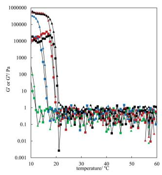
Fig. 3 Variation of G' (triangles) and G'' (squares) with temperature for HOSO gels containing different concentrations of MA ((green-4 wt%, blue-5 wt%, red-6 wt%, black-7 wt%)) upon cooling from 80 °C at 1 °C min<sup>-1</sup>. Measurements were made at a strain of 0.01% and a frequency of 1 Hz: data only shown from 60 °C.
