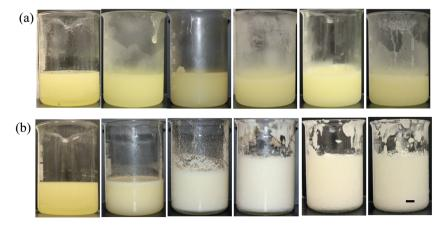
Fig. 5 Photographs of vessels containing mixtures of MA in HOSO at different concentrations (a) before aeration and (b) immediately (within 1 min) after whipping at 22  $^{\circ}$ C. MA concentrations in wt% are (left to right) 2.0, 3.5, 4.5, 5.0, 6.0 and 10.0. The sample at 2.0 wt% is one-phase, all other samples are two-phase. Scale bar = 1 cm.
