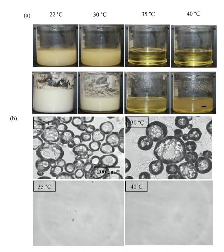
Fig. 9 (a) Appearance of vessels containing 8 wt% MA in HOSO before (upper) and after (lower) whipping at different temperatures, scale bar = 1 cm and (b) optical microscope images of mixtures after whipping for temperatures given, scale bar same in all cases.
