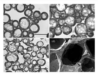
Fig. 7 (a)–(c) Optical microscopy images of air-in-HOSO foams prepared at 22  $^{\circ}$ C and stabilised by crystals of MA at concentrations of (a) 5 wt%, (b) 7 wt% and (c) 8 wt%. Scale bars = 200  $\mu$ m. (d) Cryo-SEM image of an oil foam formed at 22  $^{\circ}$ C containing 10 wt% MA.
