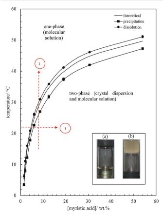
Fig. 1 Variation of MA solubility in HOSO with temperature, with points obtained from cooling at 0.1 °C min<sup>-1</sup> (squares) and heating at 0.1 °C min<sup>-1</sup> (circles). The full line without points is that calculated using eqn (1). Inset: photographs of (a) oil solution, upright at 40 °C, and (b) oil gel, inverted at 22  $^{\circ}\text{C},$  for 10 wt% MA. Routes 1 and 2 are those followed during aeration (later).
