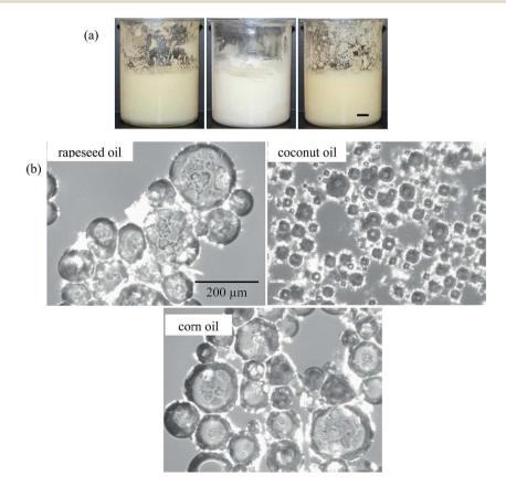
Fig. 11 (a) Appearance of air-in-oil foams after whipping 5 wt% MA in oil at 22 °C for rapeseed oil (left), coconut oil (middle) and corn oil (right), scale bar = 1 cm and (b) corresponding optical micrographs, scale bar same in all cases.
