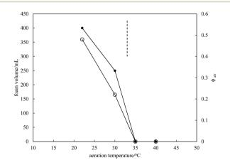
Fig. 10 Variation of foam volume produced (filled points) and volume fraction of air in foam (unfilled points) *versus* aeration temperature for 8 wt% MA in HOSO. Mixtures originate from the two-phase region to the left of the dashed line and from the one-phase region to the right of it.
