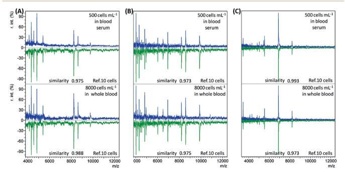
Fig. 2 Immunoaffinity MALDI-TOF mass spectra (in blue) for a low concentration of (A) *E. coli*, (B) *B. subtilis*, and (C) *S. aureus* in blood serum (500 cells per mL) or whole blood (8000 cells per mL), and comparisons with the reference spectra (in green) of the corresponding species at 10 cells with similarity scores calculated using the cosine correlation method (r.int: relative intensity).
