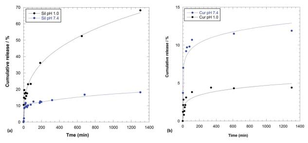
Fig. 8 Amount of (a) silibinin and (b) curcumin released from 1 in 0.1 M HCl solution and phosphate buffer pH 7.4.
