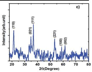
Fig. 2 (a) FESEM image of the  $\alpha$ -FeO(OH) nanowires, (b) SEM image of the Ni doped FeO(OH)-NWs-AC and (c) XRD pattern of the prepared  $\alpha$ -FeO(OH) nanowires.
