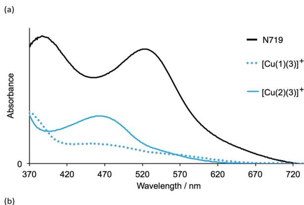
**Fig. 4** (a) Photographs of the electrodes. (b) Solid-state absorption spectra of  $\text{TiO}_2$  functionalized with  $[\text{Cu}(1)(3)]^+$ ,  $[\text{Cu}(2)(3)]^+$  or N719. Spectra were background-corrected by subtraction of the absorption spectrum of a blank electrode, then normalized for zero absorption at 800 nm.
