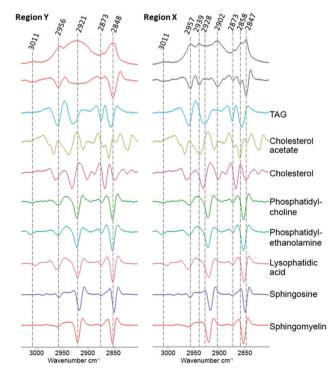
**Fig. 4** Comparison of the FTIR spectra from the CH stretching region (2750–3020 cm<sup>-1</sup>) extracted from region X and region Y (Fig. 2D) with second derivative spectra shown below followed by a range of pure lipid spectra as assigned.
