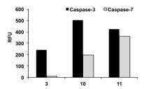
Fig. 2 Comparison of fluorescence increase ( $\lambda_{Ex/Em}$  485/525 nm) with substrates **3** (Asp-Glu-Pro-Asp-Ahx), **10** (Asp-Glu-Pro-Asp-Ser-Ahx) and **11** (Asp-Glu-Val-Asp-Ser-Ahx) at 3.1  $\mu$ M (n=3, standard deviation  $\pm 1.0-3.1$  RFU) incubated with caspase-3 and caspase-7 (15 nM) for 60 min.
