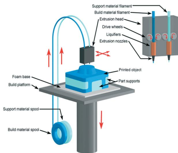
**Fig. 17** Schematic illustration of FDM 3D printer. The feedstock filament of thermoplastic material is drawn from a spool into the FDM extrusion head, in which it is heated into a semiliquid state and then by drive wheels it is extruded out through nozzle on a built platform.<sup>20</sup> (Copyright 2008 Custom Part Net).
