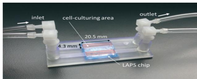
Fig. 10 LAPS chip with attached microfluidic channels.<sup>54</sup> (Copyright 2015 WILEY).
