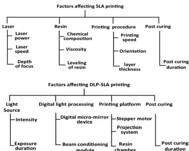
**Fig. 8** Parameters affecting laser and DLP-SLA print process.
