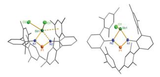
Fig. 6 Molecular structure of 2a (left) and 3 (right). Thermal ellipsoids are drawn at 50% probability (173 K). Selected bond lengths [Å] and angles [°]: 2: Sb1-N1 2.133(4), Sb1-N2 2.392(4), Sb1-Cl1 2.358(2), Sb1-Cl2 2.451(2), P1-N1 1.623(4), P1-N2 1.598(4), N2-P1-N1 96.0(2). 3: Sb1-N1 2.136(3), Sb1-N2 2.171(3), Sb1-Cl1 2.342(1), P1-N2 1.625(3), P1-N1 1.643(4), N2-P1-N1 91.7(2).
