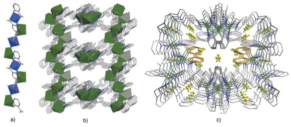
Fig. 11 (a) Formation of metal chains in  $\{[Zn_2(nica)_2(bpy)_{1.5}(H_2O)] \cdot 0.5(bpy) \cdot 3H_2O\}_n$  through coordination of nica<sup>2-</sup> (H<sub>2</sub>nica = nicotinic acid) ligands in a chelating manner; (b) the 3D framework in  $\{[Zn_2(nica)_2(bpy)_{1.5}(H_2O)] \cdot 0.5(bpy) \cdot 3H_2O\}_n$  viewed along the c-axis; (c) incorporation of guest molecules such as water and 4,4'-bipyridine. Adapted from ref. 77 with permission from © 1996-2016 MDPI AG.
