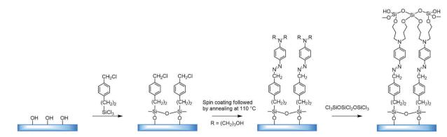
Fig. 7 Formation of a non-centrosymmetric multilayer of a film by combining self-assembly and a surface reaction of S<sub>N</sub>2 type. Adapted from ref. 28 (with permission from Copyright © 2016 American Chemical Society)
