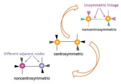
Fig. 21 Two methods for removing an inversion center in a diamondoid structure: (top) using unsymmetrical linkage and (below) using different adjacent nodes. Adapted from ref. 80 (Copyright © 2012, American Chemical Society).
