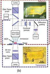
Fig. 9 (a) Schematic representation of the Kurtz method for powders. (b) Confocal multifunctional micro-spectroscopy setup for precision optical measurements with a single crystal of a MOF. The upper and lower channels are for reflectance and transmission measurements that can be upgraded to simultaneous luminescence measurements. Copyright Royal Society of Chemistry
