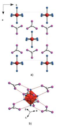
Fig. 23 Representation of the non-centrosymmetric structure of  $[C(NH_2)_3]_2[TiF_6]$ ; (a) in the ab plane; and (b) showing the F···H bonds. Adopted from ref. 110 (Copyright © 2011 Elsevier Inc).
