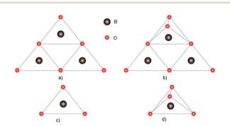
Fig. 4 Structural units that make up borate crystals: (a) B<sub>3</sub>O<sub>6</sub>, (b) B<sub>3</sub>O<sub>7</sub>, (c) BO<sub>3</sub>, and (d) BO<sub>4</sub>. Adapted from ref. 10 (with permission from Copyright © Royal Society of Chemistry 2016).
