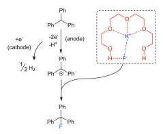
Scheme 13 Schematic representation of electrochemical fluorination
