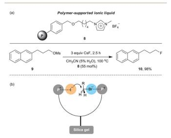
Scheme 5 (a) Application of polymer-supported IL  ${\bf 8}$  in a fluorination reaction. (b) Bicipital effect of neighboring ion pairs using a polymer-supported phosphonium salt.
