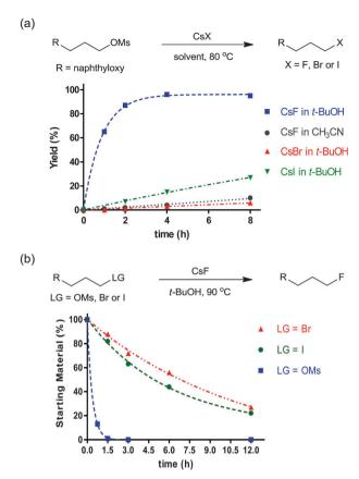
Fig. 5 (a) Reactivity of CsF, CsBr, and CsI in t-BuOH or CH<sub>3</sub>CN. (b) Unusual leaving group ability in the t-BuOH reaction medium.
