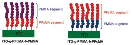
Scheme 15 Variation of the distance between PFcMA and the electrode (ITO) in surface bonded block-copolymers. Reprinted with permission from ref. 10. Copyright (2010) American Chemical Society.
