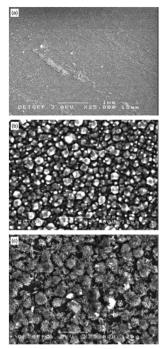
Fig. 24 SEM of films grown from AACVD deposition of InMe<sub>3</sub> and MeOH at (a) 400 °C; (b) 450 °C; and (c) 500 °C. Reproduced with permission from ref. 176 Copyright 2013 Royal Australian Chemical Institute
