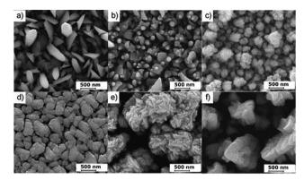
Fig. 3 SEM images of CdS thin films deposited from  $[Cd(S_2CNCy_2)_2 \cdot py]$  on FTO (a–c) and soda glass (d–f) at 350, 400, and 450 °C from THF solution. Reproduced with permission from ref. 37. Copyright 2012 Wiley.
