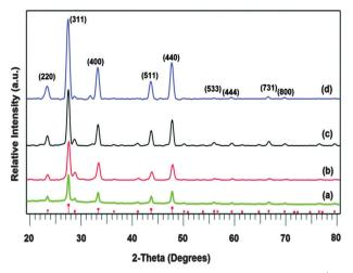
Fig. 6 p-XRD patterns of as deposited  $In_2S_3$  thin films from  $In[(S_2P^iBu_2)_3]$  precursor at temperatures (a) 350 °C, (b) 400 °C, (c) 450 °C and (d) 500 °C. Vertical lines below show the standard ICDD pattern 01-084-1385 for  $In_2S_3$ . Reproduced from ref. 82 with permission from the Centre National de la Recherche Scientifique (CNRS) and the Royal Society of Chemistry.
