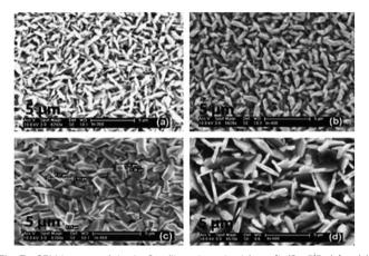
Fig. 7 SEM images of the  $In_2Se_3$  films deposited from  $[In(Se_2P^jPr_2)_3]$  at (a) 300 °C, (b) 350 °C, (c) 400 °C and (d) 450 °C. Reproduced with permission from ref. 83. Copyright 2014 Elsevier.
