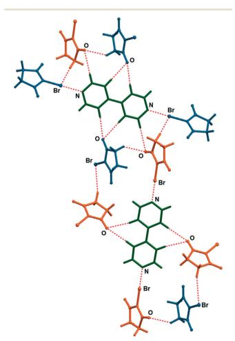
Fig. 4 Network of halogen and hydrogen bonded molecules in the crystal structure of (nbs)2(bpy).
