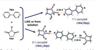
**Fig. 1** Structures of reactants, *N*-bromosuccinimide (**nbs**) and 4,4-bipyridine (**bpy**), and the cocrystal structures obtained as a result of the single crystal X-ray diffraction experiment.
