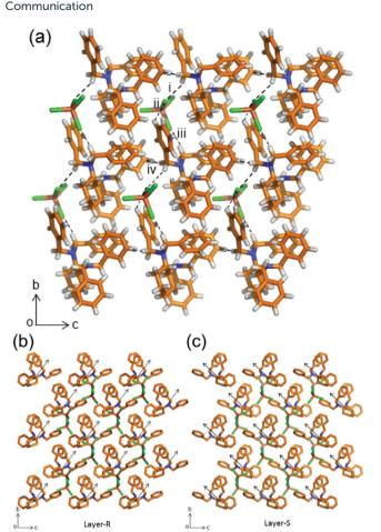
**Fig. 3** Crystal structure of the β-phase viewed along *a*-axis formed by C-H···Cl interactions among [HL]<sup>+</sup> cations and [FeCl<sub>4</sub>]<sup>-</sup> anions and repulsive C-H···H-C intermolecular interactions. The hydrogen bonding interactions are shown with a dashed black line (a). Packing of half a unit cell (*a*-axis) showing the non-centrosymmetric and polar orientation (black arrows) of layers of the enantiomers R (b) and S (c). Color code as in Fig. 1.
