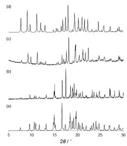
Fig. 4 The simulated isotropic XRPD patterns of  $\beta$  (a) and  $\alpha$  (d) phases calculated from single crystal structures. Experimental XRPD pattern corresponding to the  $\beta$  phase at room temperature (b) and that of the  $\beta$  phase at 110 °C measured *ex situ* at room temperature (c).
