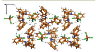
Fig. 2 Crystal structure of the  $\alpha$ -phase viewed along the a-axis showing the various C-H···Cl interactions among [HL]<sup>+</sup> cations and [FeCl<sub>4</sub>]<sup>-</sup> anions. The hydrogen bonding interactions are shown with a dashed black line. Color code as in Fig. 1.
