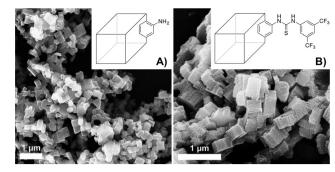
Fig. 8 SEM images of nanoscale A) IRMOF-3 and B) IRMOF-3thiourea-3,5-(CF<sub>3</sub>)<sub>2</sub>Ph derivative. Reprinted with permission from ref. 56. Copyright ® Royal Society of Chemistry.
