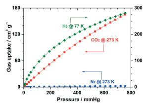
Fig. 7 Gas sorption isotherms of Cu-UBTA for  $CO_2$  and  $N_2$  (at 273 K), and  $H_2$  (at 77 K). Reprinted with permission from ref. 55. Copyright ® Royal Society of Chemistry.
