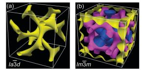
Fig. 4 Reconstructed EDMs: (a) of a unit cell of the Cub/ $la\bar{3}d$  phase of **AB8** only showing the high density regions and (b) of the  $lm\bar{3}m$  approximate of the Cub $^{[x]}/l432$  phase of **AB14** showing the three distinct iso-surfaces with different colour.
