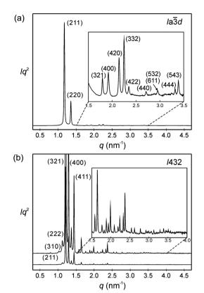
**Fig. 3** SAXS diffractograms of (a) the Cub/ $la\bar{3}d$  phase ( $a_{\rm cub}=13.10$  nm) of **AB8**, recorded at T=150 °C on heating (for wide angle scattering see Fig. S10b, ESI†); (b) the Cub $^{\rm l*}$ //432 phase ( $a_{\rm cub}=19.46$  nm) of **AB14** at T=140 °C, the curve on top is enhanced by a factor of 7 and only some diffractions at lower angles are labelled; see also Tables S3–S6 (ESI†).
