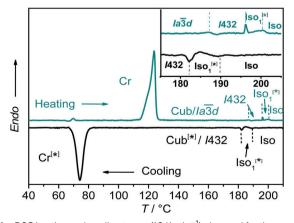
Fig. 1 DSC heating and cooling traces (10 K min<sup>-1</sup>) observed for the complex AB8. The inset shows the heating and cooling traces for the temperature range of the Iso-Iso<sub>1</sub>[\*]-Cub<sup>[\*]</sup>//432 transitions between 175 °C and 205 °C.
