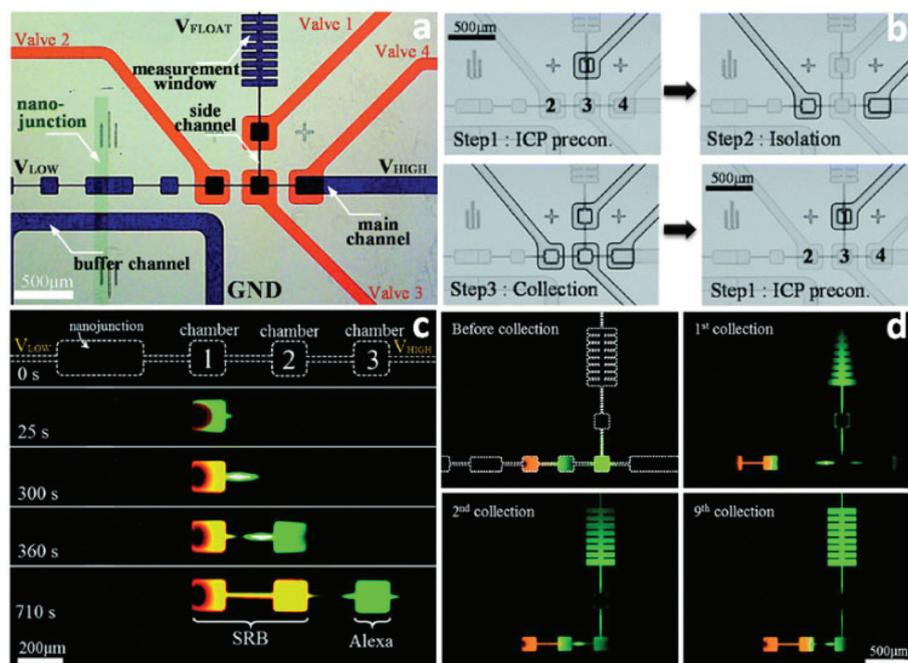
**Fig. 5** Schematic illustration of the mTAS using ICP and microvalves. (a) Microscopic view of the device (the microchannels in the ICP layer were indicated with blue and the microchannels in the valve layer were indicated red); (b) depiction of the three-step microvalve control; (c) time-lapse images of the simultaneous preconcentration and separation of SRB and Alexa; (d) snapshots of the repeated valve operations for collecting Alexa dye.
