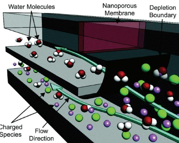
**Fig. 6** Depiction of the out-of-plane desalting device. The green plane indicates the boundary of the IDZ formed by the Nafion membrane at the intersection of the desalted (upper) and brine (lower) streams. By stacking these streams and the ground (auxiliary) channel vertically, the authors achieved greater functional density than can be obtained in a planar device.
