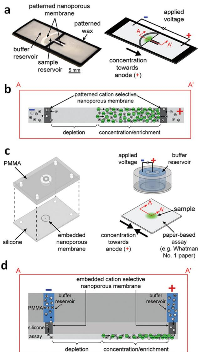
**Fig. 3** Design and operation of the external and in-paper devices for concentration. (a) Schematic of the in-paper transport configuration. (b) Cross-section of the in-paper devices illustrating ICP under an applied voltage. (c) Schematic of the external concentration device. (d) Cross-section of the devices and paper-based assays depicting ICP under an applied voltage. (Image reproduced from ref. 11 with permission. Copyright 2016, American Chemical Society.)
