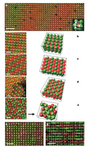
Fig. 7 CsCl-type binary crystals formed from oppositely charged colloids. All particles were dispersed in salt-containing CHB-decalin solutions. In subfigures (a-e), red particles are positive PMMA latexes and green particles are negative PMMA latexes; in subfigures (f and g), green particles are positive PMMA latexes and red particles are negative silica. Reprinted by permission from Macmillan Publishers Ltd: Nature, Leunissen et al., 2005.33
