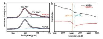
Fig. 2 (a) Normalized O 1s core-level XPS and (b) EPR spectra collected for  ${\rm Nb_2O_5}$  and  ${\rm Nb_2O_{5-x}}$  NPs films.
