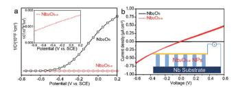
Fig. 3 (a) Mott–Schottky plots of  $Nb_2O_5$  and  $Nb_2O_{5-x}$  NPs films at a frequency of 1 kHz in the dark; (b) comparison of I-V curves of the samples; the inset is the schematic of the measurement.
