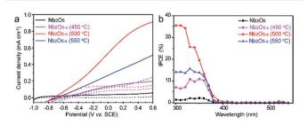
Fig. 4 (a) I-V curves measured under 100 mW cm $^{-2}$  simulated solar light generated by a 100 W xenon lamp coupled with an AM 1.5G filter in 1 M NaOH electrolyte; (b) IPCE spectra measured at 0.2 V vs. SCE in 1 M NaOH electrolyte.
