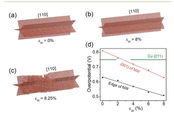
Fig. 6 (a-c) The atomic structure of the penta-twinned Cu NW under  $\varepsilon_{zz}=0\%$ , 8% and 8.25%. Only the twin boundaries and other lattice defects are shown. (d) Overpotential on the NW edge and (001) facet as functions of uniaxial tension  $\varepsilon_{\rm zz}$ . The green horizontal line indicates the overpotential on the Cu (211) surface
