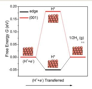
Fig. 4 The free energy diagrams of the HER on the NW edge and (001) facet.
