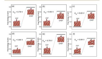
5 The overpotential-determining step as a function of H configuration on the NW. (a) A single H atom on the edge and the 1st NN to the adsorbed CO; (b) a single H atom on the facet and the 1st NN to CO; (c) a single H atom on the facet and the 2nd NN to CO; (d) a single H atom on the edge and the 2nd NN to CO; (e) one H on the facet and another H on the edge; both are 1st NNs to CO; (f) two H atoms on the facet and the 1st NNs to CO.
