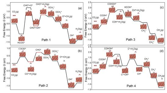
Fig. 2 The free energy diagrams for the formation of CH<sub>4</sub> on the NW edge.
