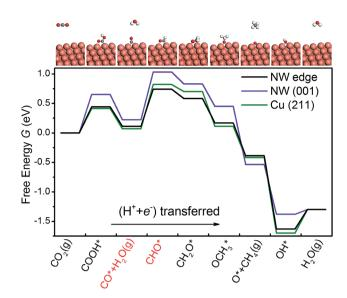
Fig. 3 The free energy diagrams of  $CO_2$  electroreduction on the NW edge, the NW (001) facet and the Cu (211) surface at 0 V vs. RHE. The two intermediates shown in red indicate the overpotential-determining step. The large orange spheres represent Cu atoms, and the small spheres represent O (red), C (gray) and H (white) atoms.
