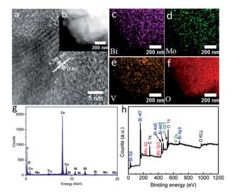
Fig. 3 (a) The HETEM image, (b) HAADF-STEM image, elemental mapping images of (c) Bi, (d) Mo, (e) V and (f) O, (g) EDX spectrum and (h) the survey XPS spectrum of  $BiMo_{0.015}V_{0.985}O_4$ .
