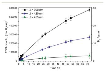
Fig. 2 Photocatalytic  $H_2$  production with Dmb [NiFeSe]– $H_2$ ase (50 pmol) with  $CN_x$ – $TiO_2$  (5 mg) in EDTA (pH 6, 0.1 M, 3 mL) under AM 1.5G irradiation at an intensity of 1 Sun at  $\lambda$  > 300, 420 and 455 nm.
