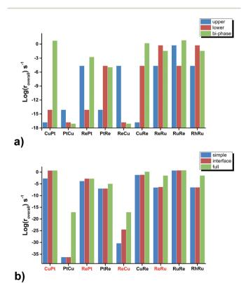
Fig. 3 Activity ( $log(r_{overall})$ ) comparisons of nine bi-phase surfaces among (a) those from the upper phase, lower phase and bi-phase surfaces, respectively, (b) the simple, interface and full kinetic models, where the reactive-noble bi-phase surfaces are highlighted in red.
