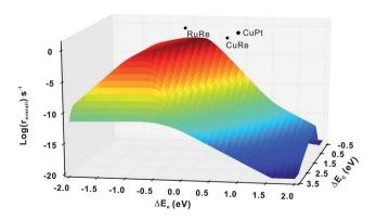
Fig. 4 Comparison of activities ( $log(r_{overall})$ ) between the mono-phase volcano surface and the three bi-phase surfaces, RuRe, CuRe and CuPt, illustrating that some bi-phase systems can achieve activities far beyond the mono-phase volcano surface.
