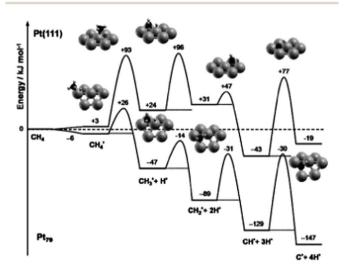
Fig. 13 ZPE-corrected reaction energy profile for the complete dehydrogenation of methane on a Pt(111) surface and on a Pt $_{79}$  nanoparticle. All energies, in kJ  $\mathrm{mol}^{-1}$ , refer to methane in the gas phase and the clean substrate. Reprinted with permission from ref. 59. Copyright 2010 Wiley-VCH Verlag GmbH.
