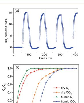
Fig. 5 (a)  $CO_2$  adsorption–desorption cycling curve for 1-dmen in humid conditions. (b) Breakthrough curves for 1-dmen under dry ( $N_2$ , red circle;  $CO_2$ , orange circle) and humid conditions ( $N_2$ , green triangle;  $CO_2$ , blue triangle).
