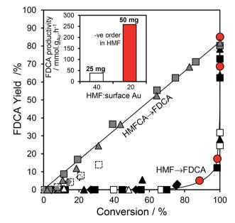
Fig. 5 (main) Disparate evolution of FDCA yield as a function of either HMF or HMFCA conversion over 25 mg △(△) 0.5 wt%, ◆(♠) 1 wt%, □(□) 2 wt%, □(□) 5 wt%, and ▲(♠) 10 wt% Au/HT catalysts, and 50 mg ● 2 wt% Au/HT; (inset) normalised FDCA productivity per Au atom as a function of HMF: surface Au molar ratio for 2 wt% Au/HT highlighting self-poisoning by high HMF concentrations.
