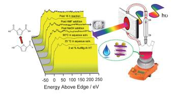
Fig. 3 Operando Au  $L_{\rm III}$ -edge XAS of a 2 wt% Au/HT catalyst during aqueous phase selective aerobic oxidation of HMF; catalytically active, metallic gold nanoparticles are unaffected by hot water or NaOH addition.
