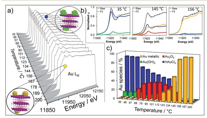
Fig. 1 In situ Au  $L_{III}$  XANES during thermal processing of the HAuCl<sub>4</sub>/Mg-Al HT precursor: (a) thermal evolution of normalised XANES spectra; (b) representative least squares fitted XANES spectra to reference gold species; (c) quantitative thermal evolution of fitted Au species.
