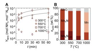
Fig. 6  $\,$  NH $_3$  evolution via isothermal transition-metal nitride reduction: (A) NH $_3$  yield vs. time and (B) solid weight fractions from the reaction of Mn $_4$ N with H $_2$  at 1 bar vs. temperature. Error bars are via error propagation within a 95% confidence interval. Solid lines are shrinking-core models for the data at 550 °C and 700 °C controlled by the chemical reaction or gas phase diffusion.
