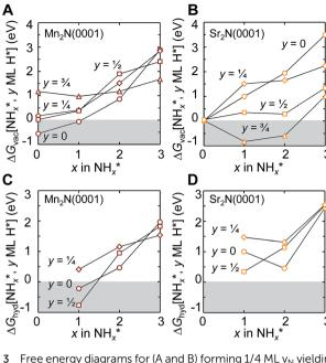
Fig. 3 Free energy diagrams for (A and B) forming  $1/4 \text{ ML } v_N$  yielding  $1/4 \text{ ML } NH_x^*$  and (C and D) hydrogenating  $NH_{x-1}^*$  to  $NH_x^*$  and y=0 (circles), 1/4 (diamonds), 1/2 (squares), and 3/4 (triangles) ML  $H^*$  adatoms on (A and C)  $Mn_2N(0001)$  and (B and D)  $Sr_2N(0001)$  at  $25\,^{\circ}\text{C}$  and 1 bar. Lines are a guide only. The shaded regions mark energetically favourable surface reactions.
