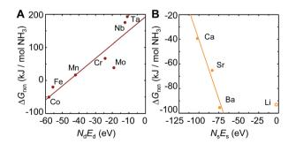
Fig. 2 Scaling of the free energy of the  $NH_3$  evolution at 25 °C (computed from tabulated free energy data as described in Section 3.1) via metal nitride (A) reduction and (B) hydrogenation with the product of the number of electrons in the metal ground state, N, and the energy of these electrons, E, in the (A) d-states and (B) s-states. The metal marks the metallic constituent of the composition given with ESI.† Solid lines are fits to the data shown with solid symbols.
