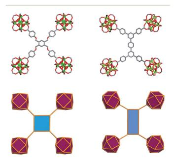
Fig. 5 Illustration of the ligand geometry effect on the orientation of the 12-c cluster in ftw-fragment of ftw-MOF-1 (left) and ftw-MOF-2 (right).11
