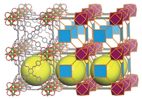
Fig. 4 Molecular and vertex figure representation of ftw-MOF-1, yellow spheres denote the open space within each cage; (top left) TetPOMB ligand coordinated to four 12-connected hexanuclear clusters and (bottom right) vertex figure representation.11
