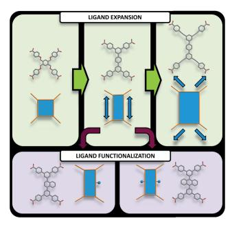
Fig. 3 Pathways to modify quadrangular ligands for the synthesis of ftw-MOFs, including examples of ligands and their vertex figures. (Top) Modification of the organic quadrangular MBB through ligand expansion. (Bottom) Modification of the quadrangular organic MBB through ligand functionalization.
