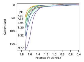
Fig. 5 CV of 0.25 mM  $[Ru(Py_3PO)(bpy)(OH_2)]^{2+}$  at pH 7.00 (red), 7.35 (yellow), 7.95 (green), 8.30 (teal), 9.32 (blue), and 9.77 (purple) at 100 mV s<sup>-1</sup>. Conditions: 0.1 M phosphate, 3 mm glassy carbon working electrode, Pt wire counter electrode, Ag/AqCl reference electrode.
