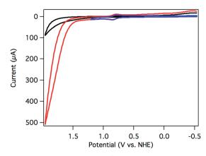
Fig. 3 CV of  $[Ru(Py_3PO)(bpy)(OH_2)]^{2+}$  (3) swept anodically to 1.95 V (red) and 1.2 V (blue) vs. NHE. A catalyst-free background scan is shown in black. The reduction near -0.5 V is assigned to  $O_2$  reduction. Conditions: 250 mV s<sup>-1</sup> scan rate, pH 7 0.1 M phosphate buffer, 3 mm glassy carbon disk working electrode, Pt wire counter electrode, Ag/AqCl reference electrode.
