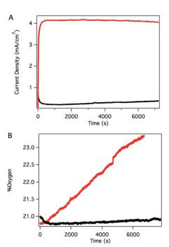
Fig. 4 (A) Controlled potential electrolysis (CPE) of solutions containing 3 (red) and without catalyst (black) at 1.8 V  $\nu$ s. NHE. (B) Headspace O $_2$  fluorescence detection during CPE of solutions containing 3 (red) and without catalyst (black). Conditions: 0.45 mM catalyst, 0.1 M phosphate at pH 7, 1.4 cm $^2$  planar ITO electrode.
