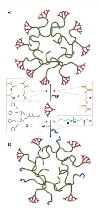
Fig. 1 Schematic representation of idealised hyp-polydendron synthesis. Atom transfer radical copolymerization (ATRP) of 2-hydroxypropyl methacrylate, 2, and ethylene glycol dimethacrylate, 3, initiated by the functional  $G_2$  dendron, 1 to form (A) hyp-polydendrons; and (B) inclusion of a PEG<sub>16</sub>-initiator, 4, to form hyp-polydendrons with controlled and mixed surface functionality.
