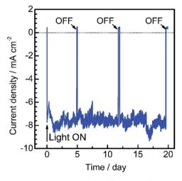
Fig. 4 Current–time curve for a Pt/CdS/CuGa $_3$ Se $_5$ /ACGSe electrode with CuGa $_3$ Se $_5$  deposited for 15 min at a potential of 0 V<sub>RHE</sub>. A buffer solution of 0.05 M Na $_2$ HPO $_4$  + 0.05 M NaH $_2$ PO $_4$  (adjusted to pH 7 by addition of NaOH) was used as the electrolyte. 420–800 nm light (100 W cm $^{-2}$ ) from a Xe lamp equipped with a cutoff filter (HOYA, L42) and a cold mirror (Optline, CM-1) was employed as the light source.
