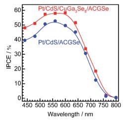
Fig. 2 Wavelength dependence of the IPCE spectra for Pt/CdS/CuGa $_3$ Se $_5$ /ACGSe with CuGa $_3$ Se $_5$  deposited for 15 min, and Pt/CdS/CGSe measured at an applied potential of 0 V $_{\rm RHE}$ . The IPCE was measured in 0.1 M Na $_2$ HPO $_4$  (adjusted to pH 10 by addition of NaOH) under monochromatic light from a 300 W Xe lamp equipped with band-pass filters and an optical fiber.
