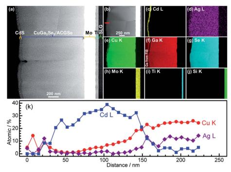
Fig. 7 Cross-sectional TEM images of CdS/CuGa $_3$ Se $_5$ /ACGSe sample with CuGa $_3$ Se $_5$  deposited for 15 min (a) and (b); EDX elemental maps for Cd (c), Ag (d), Cu (e), Ga (f), Se (g), Mo (h), Ti (i), Si (j); and line profiles for Cd, Cu and Ag across the CdS and CuGa<sub>3</sub>Se<sub>5</sub>/ACGSe interfaces (k). The red line in Fig. 4b indicates where the linear profile was measured. The sample was sliced using a Ga focused ion beam (FIB).
