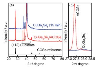
Fig. 5 XRD patterns for  $CuGa_3Se_5/ACGSe$  with  $CuGa_3Se_5$  deposited for 15 min, and a reference  $CuGa_3Se_5$  film deposited on Mo/Ti/SLG for 15 min (a), and the corresponding (112) diffractions (b). The reference pattern for CGSe (PDF no. 31-456) is shown at the bottom for comparison.
