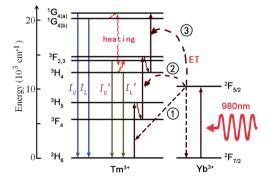
Fig. 6 The mechanism of optical thermal sensing through  $Yb^{3+}-Tm^{3+}$  energy transfer under 980 nm infrared excitation.
