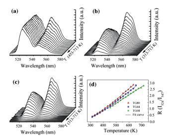
Fig. 4 Temperature dependent  $Er^{3+}$  green emission spectra of 0.5 mol%  $Er^{3+}$  doped (a)  $Te_{80}Zn_{9.5}Na_{10}$  (TG08) glass, (b)  $Te_{40}Ge_{40}Zn_{9.5}Na_{10}$  (TG44) glass, (c)  $Ge_{80}Zn_{9.5}Na_{10}$  (TG80) glass, and (d) temperature dependent R values of the two green emissions of  $Er^{3+}$ . Reprinted from ref. 21 with permission of Springer.
