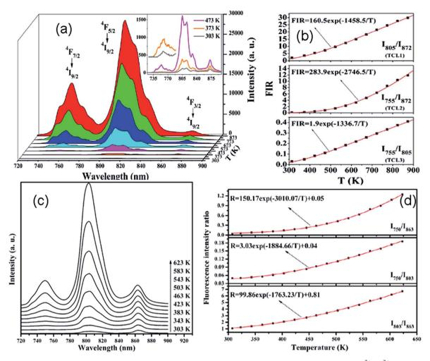
Fig. 13 Temperature dependent (a) near infrared emission spectra and (b) fluorescence intensity ratio (FIR) in  $Nd^{3+}/Yb^{3+}$  co-doped CaWO<sub>4</sub> phosphors excited by a 980 nm laser. Temperature dependent (c) near infrared emission spectra and (d) FIR in  $Nd^{3+}/Yb^{3+}$  co-doped oxyfluoride glass ceramic containing PbF<sub>2</sub> nanocrystals excited by a 980 nm laser. Reproduced from ref. 70 and 71 with permission of Optical Society of America and Elsevier.
