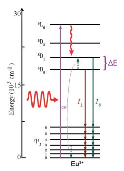
Fig. 17 The mechanism of optical thermal sensing through down-conversion of the Eu<sup>3+</sup> ion under infrared excitation.
