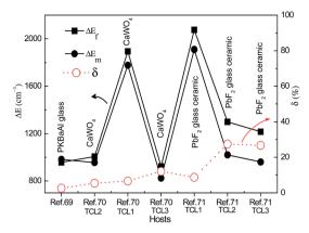
Fig. 14 Host dependent  $\Delta E_{\rm f}$  and  $\Delta E_{\rm m}$  between the TCL of Nd<sup>3+</sup> ions, and the corresponding  $\delta$  values.
