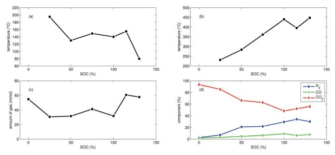
Fig. 5 Summary of all experiments with LFP cells at different SOC: (a) onset cell temperature  $\theta_{D}$ . (b) Maximum cell temperature  $\theta_{D}$ . (c) Amount of produced gas  $n_{\text{sum}}^{\text{ideal}}$ . (d) Main detected gas components  $r_i^{\text{GC}}$ .
