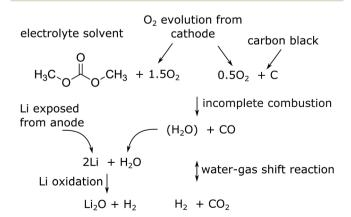
Fig. 7 Proposed main reaction system for a thermal runaway of a (partially) charged or over-charged Li-ion battery.
