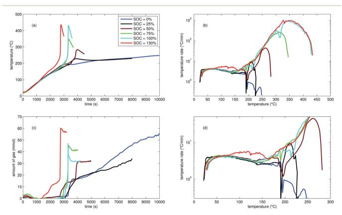
Fig. 4 Typical experiments with LFP cells: (a) cell temperature profiles. (c) Amount of produced vent-gas. (b) Cell temperature rate  $d\theta/dt$  vs. cell temperature  $\theta$ , full temperature range. (d) Close up view of the cell temperature rate.
