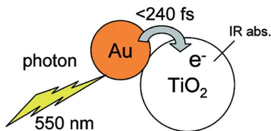
Fig. 3 Schematic representation of a gold nano dot attached on a  $\text{TiO}_2$  nanoparticle, also indicating hot electron transfer process upon the excitation of LSPR. Figure reprinted with permission from ref. 59.
