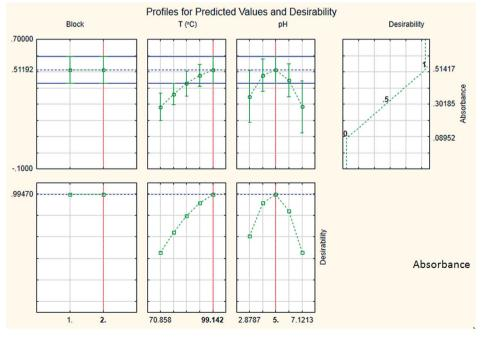
Fig. 7 Desirability function graph for CCCD.
