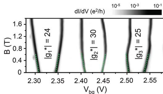
**Fig. 4** Gray scale plot of magnetic field evolution of the differential conductance  $dI_{ds}/dV_{ds}$  measured in the linear response regime (*i.e.*, at bias voltage  $V_{ds} = 0$  V) for the same quantum dot device as in Fig. 3. The  $g$  factors extracted from the measurements for quantum levels are indicated in the figure. The green dashed lines denote the data used to extract the  $g$ -factors.
