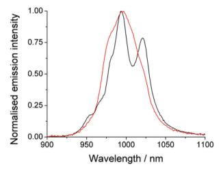
Fig. 1 Change in form of emission spectra with fluoride. Top: EuDTMA in D<sub>2</sub>O (black) and with excess sodium fluoride (red),  $\lambda_{\rm ex}$  = 394 nm, exit slit = 1 nm; inset shows the change in structure of the  $\Delta J$  = 1 band measured with 0.2 nm exit slit. Bottom: YbDTMA in D<sub>2</sub>O (black) and with added fluoride (red),  $\lambda_{\rm ex}$  = 265 nm, exit slit = 5 nm.
