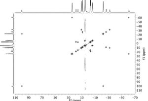
Fig. 3 Top:  $^{1}$ H NMR spectra (400 MHz, 298 K, D<sub>2</sub>O) of YbDTMA in the absence (black) and presence (red) of an excess of sodium fluoride, with assignments based on the labelled portion of the complex shown (using DyDTMA crystal structure $^{12}$ ). Bottom: EXSY spectrum of YbDTMA with fluoride at 298 K with a mixing time of 1 ms at 500 MHz.
