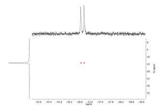
Fig. 2 <sup>19</sup>F detected <sup>89</sup>Y-<sup>19</sup>F HMQC for a D<sub>2</sub>O solution of YDTMA and excess sodium fluoride with <sup>19</sup>F on the horizontal axis and <sup>89</sup>Y on the vertical axis. The coupling in the vertical dimension is refocused during the evolution delay.
