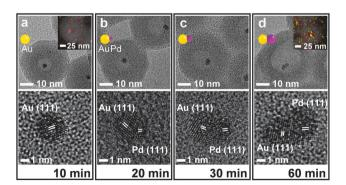
Fig. 2 TEM (upper) and HRTEM (lower) images of samples isolated during the reaction of the  $(Fe_3O_4/Au)@(SiO_2/Pd^{2+})$  with NaBH<sub>4</sub> at (a) 10, (b) 20, (c) 30, and (d) 60 min, respectively. Insets: EDX elementary maps for showing the distribution of Au (red) and Pd (yellow) elements.
