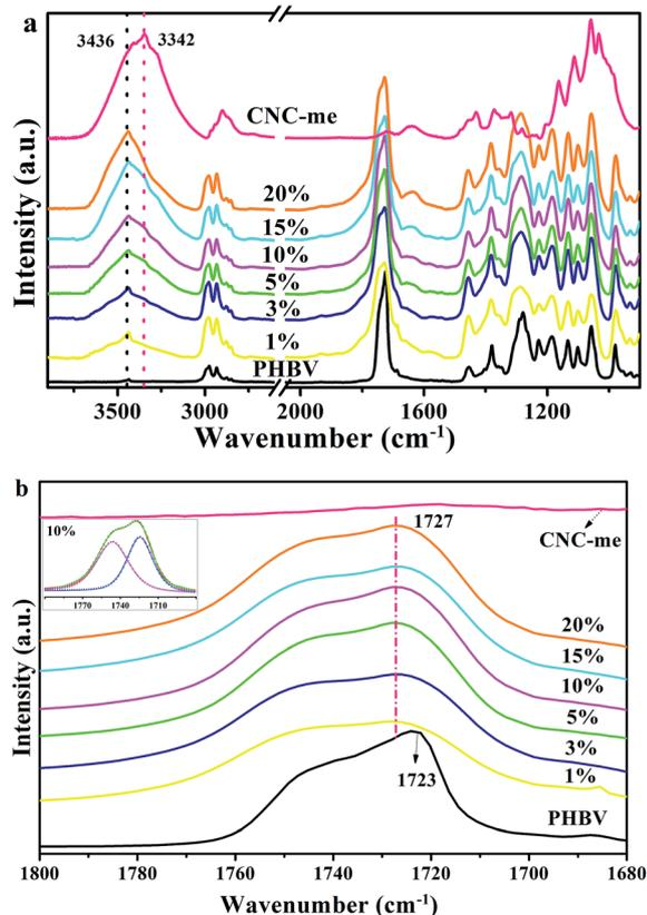
Fig. 4 FT-IR spectra (a) and carbonyl stretching region ( $\nu_{\text{C=O}}$ ) in the infrared spectra (b) for neat PHBV, CNC-me and the nanocomposites with various CNC-me concentrations and peak deconvolution for the nanocomposites with 10 wt% CNC-me (insert).
