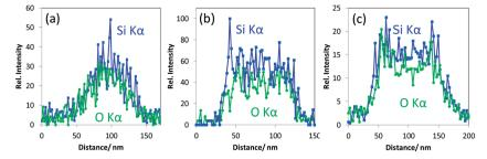
Fig. 4 Representative EDX line scans for Si K $\alpha$ , obtained on silica nanoparticles (100–150 nm diameter) classified as a) crystalline with the ordered pores therein (class one), (b) amorphous with non-ordered mesopores (class two) and (c) hollow (class three).
