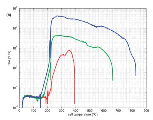
Fig. 5 (a) Overview of the time-temperature profiles for the cells tested. Data for the whole experiment durations and for the whole experiment sets is shown. For the sake of completeness, one LFP test with a higher (1) and one with a lower (2) heating rate of the heater sleeve are included. (b) Temperature rates from three representative experiments.
