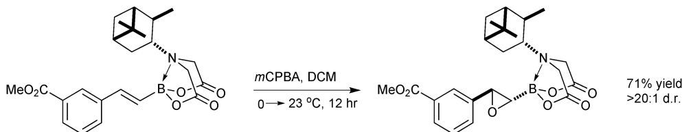
Scheme 60 Asymmetric induction from the PIDA ligand in the epoxidation of a distal alkene.
